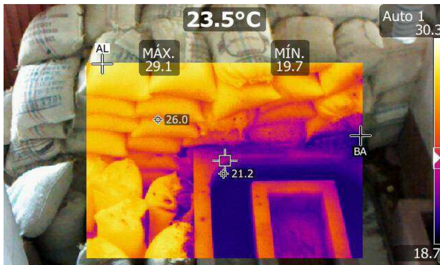
Figure 5 - Thermographic image of storage coffee in facility for coffee processing.
