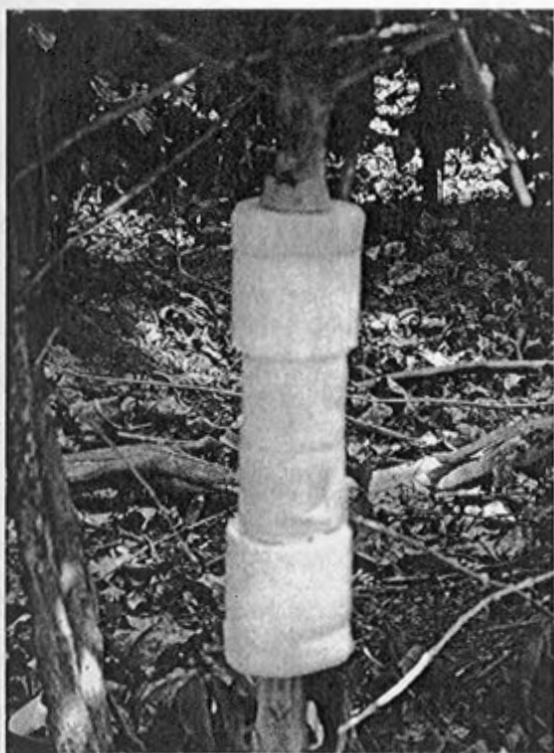
Photo 4. SGB25-ws gauge installed on a coffee trunk protected with foam collar o-rings with plastic-tack sealer on the top of the upper ring.
