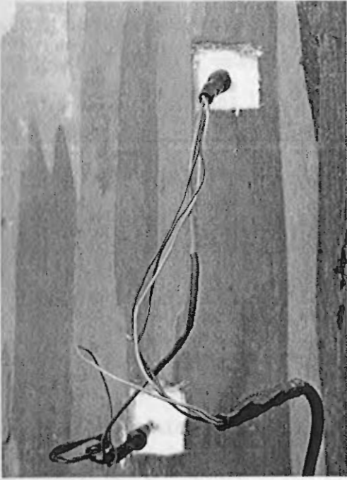
Photo 5. "Granier" probes (heated probe above, reference probe below) installed on Eucalyptus deglupta .
