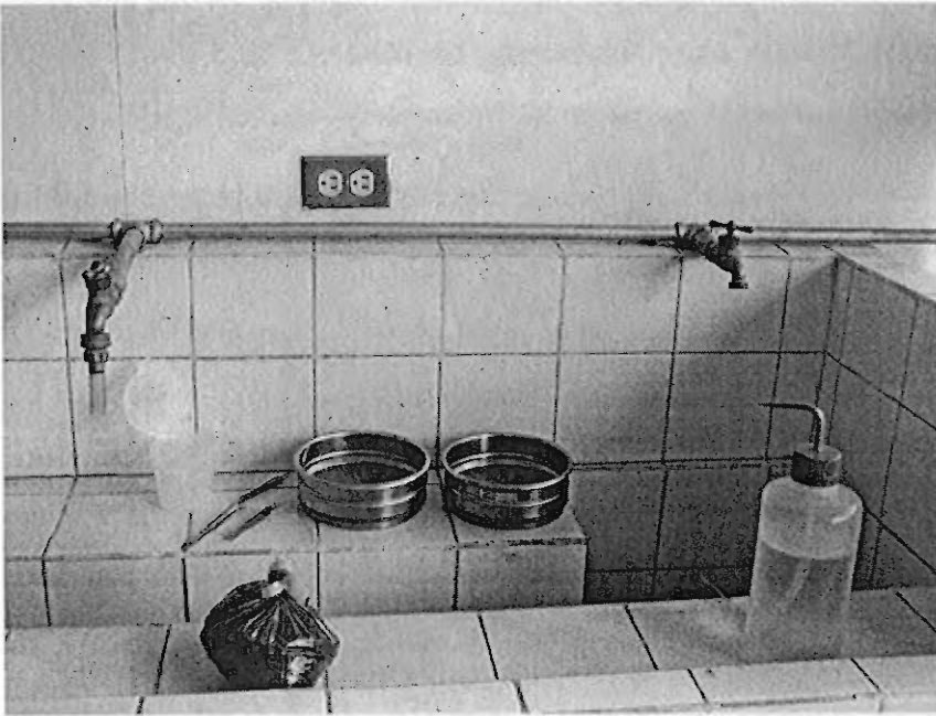
Photo 2. Root washing installation with 1.0 and 0.5 mm sieves.
