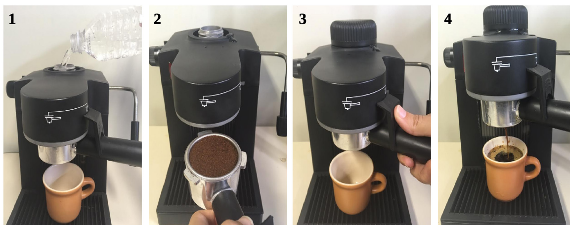
FIGURE 5 - Event sequence (1-4) for espresso coffee preparation.
