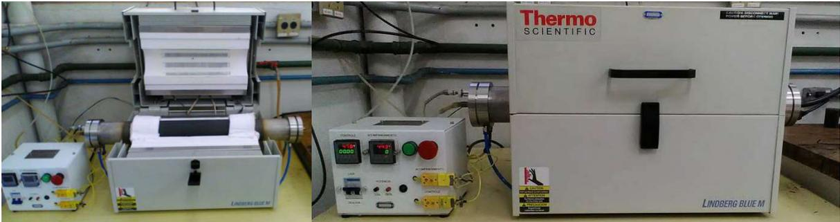
Figura 7: Imagens do reator de pirólise (Thermo Scientific Lindberg, modelo Blue M 1100C Tube Furnace).
