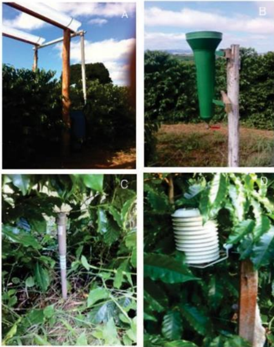
Figure 3.2 - Photographs from the Exclusion System (A) and the tools used for monitoring the environmental conditions in the experimental area: Pluviometer type Ville de Paris in an open area (B), 50-cm puncture tensiometer (C) and the thermo-hygrometer HT500 (D).
